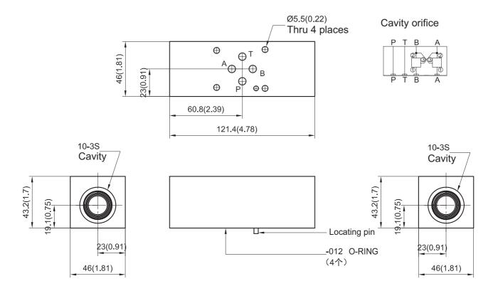
Valve torque in housing is 48-54Nm
